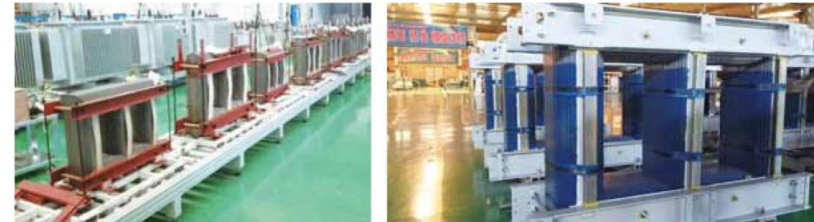
▲ 油变横向五步进叠铁芯 Oil-immersed transformer horizontal five steps laminated iron core
