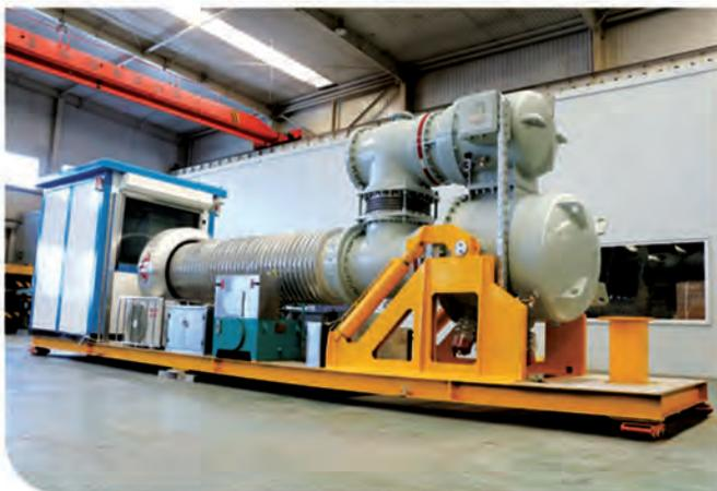
Testing device for instrument transformer measuring test
