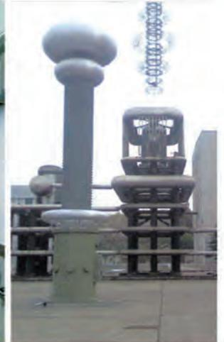
1200kV Standard vertical capacitor
