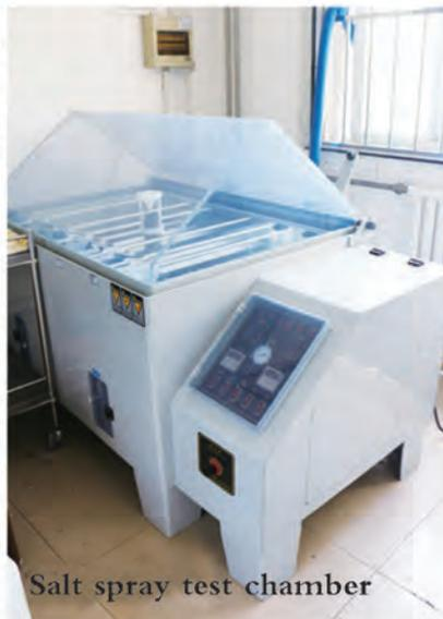
Salt spray test chamber
