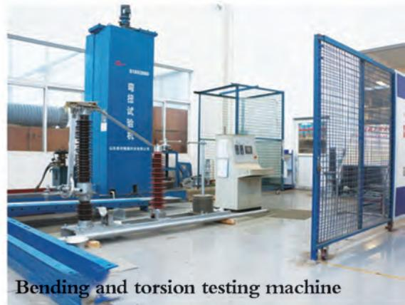
Bending and torsion testing machine
