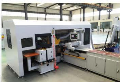
Automatic processing center for Winding Spacer, Zero burr and 0.05mm Deviation
